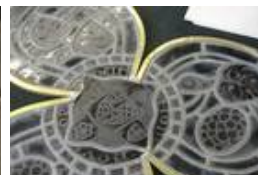
The soldered brass U-profile on another field shape
