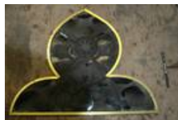
The brass frame is now circumferential and can be soldered
