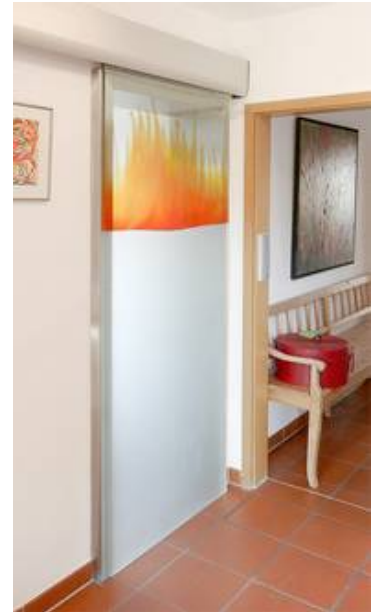
Automatic sliding glass door with affixed, hand-blown real-antique flashed glass pane in almost original size of about 900 x 640 mm and sandblasting as privacy protection in the lower area
