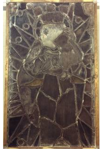
The exterior side of the medieval portrayal of the sun-crowned Madonna in reflected light displays the corrosion products typical to medieval panes.
