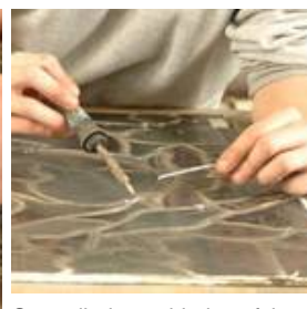
Controlled re-soldering of the broken places.
